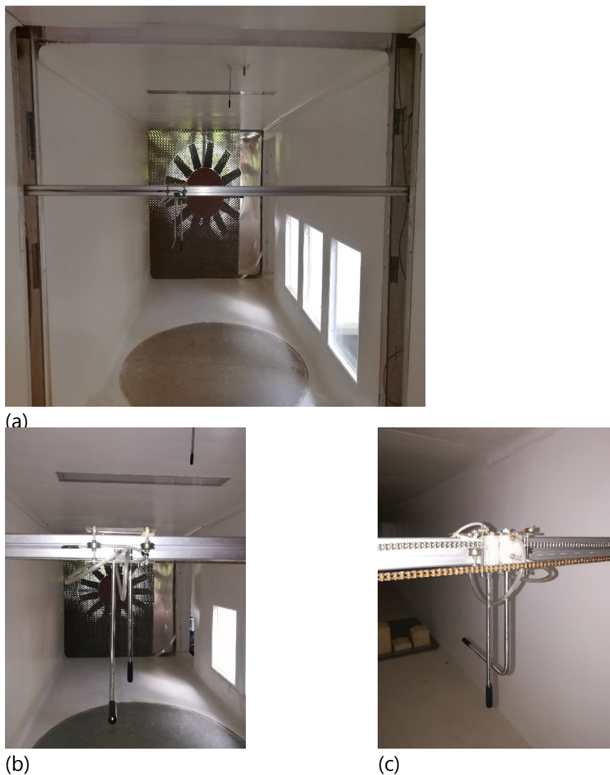
Figure 5. a) Velocity scanner, b) y c) Velocity and Pressure sensors (Pitot Tube and Hot Wire Anemometer).
